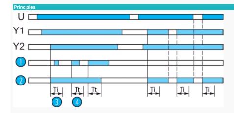
This mode is for controlling a pump based on two external signals (Y1 and Y2). The output relay closes when both input signals are present (Y1 and Y2 closed).
