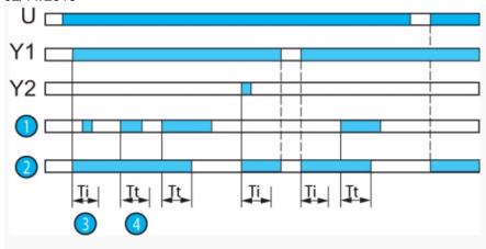
This mode is for controlling a pump based on one external signal (Y1).
